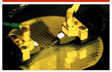
Hardware to interface with testers to develop and test semiconductors
